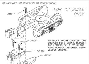
TO BODY MOUNT COUPLER, CUT COUPLER SHANK AT BOLSTER. GLUE 83059 TO BODY USING EPOXY OR AMBROID GLUE. DO NOT USE SUPER GLUE. ASSEMBLE COUPLER TO ADAPTER USING 256061 SCREWS.
